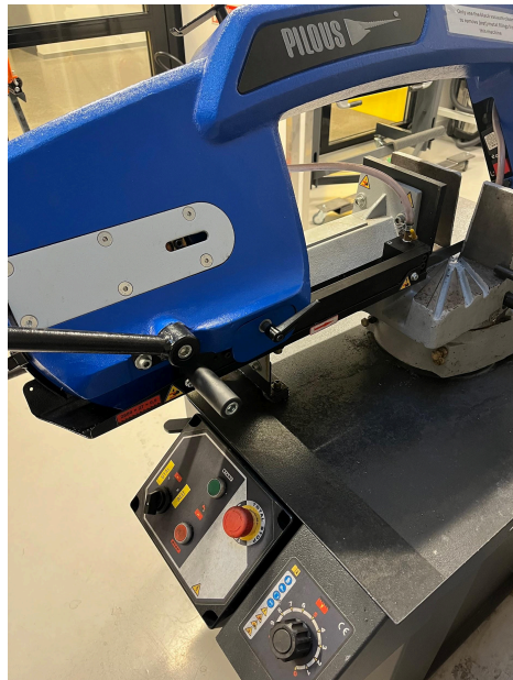
Figure 7: Blade support (black square running along blade)
