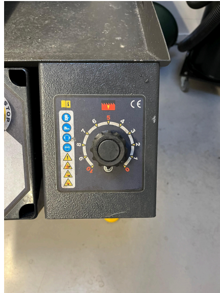
figure 2: Horizontal metal bandsaw feed rate control
