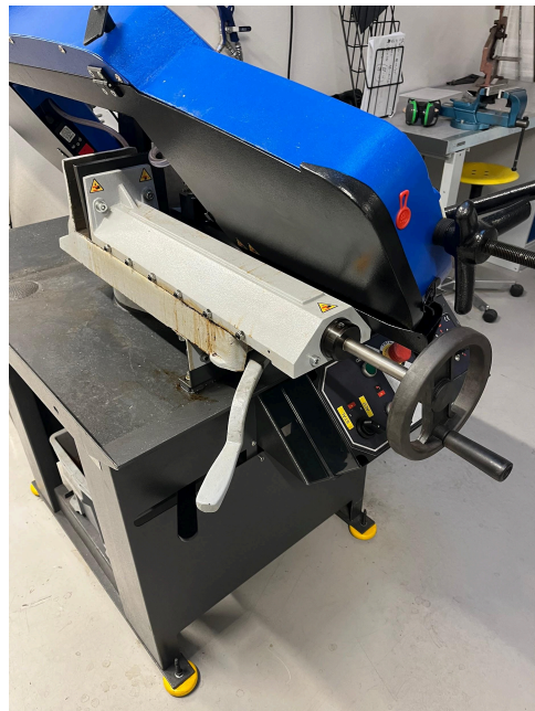
Figure 6: Horizontal band saw fast clamp lever (White closest to the camera)
