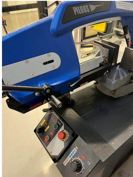
Figure 7: Blade support (black square running along blade)
