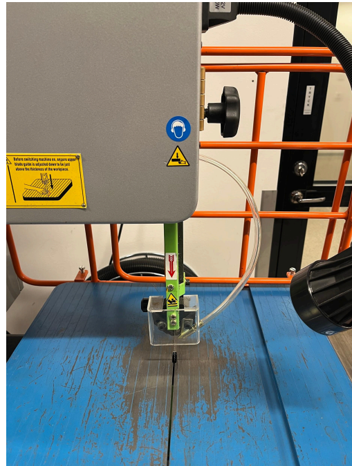
Figure 10: Blade support (Green) blade support wheel (Black above the support)
