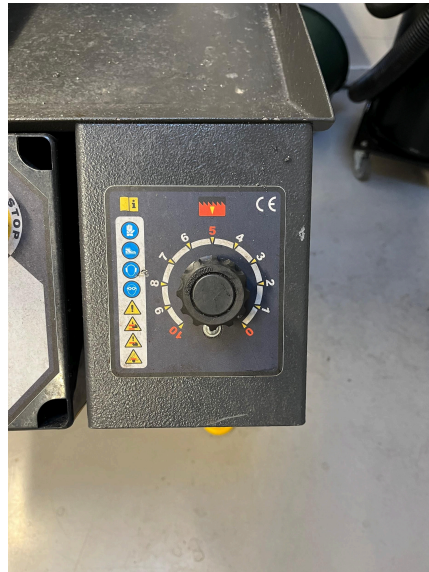
figure 2: Horizontal metal bandsaw feed rate control
